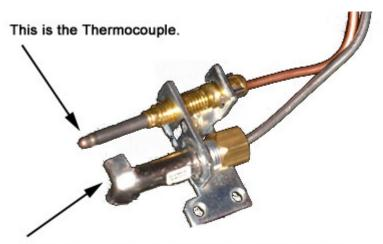
Apply flame to the end of the Pilot, using a lighter.
